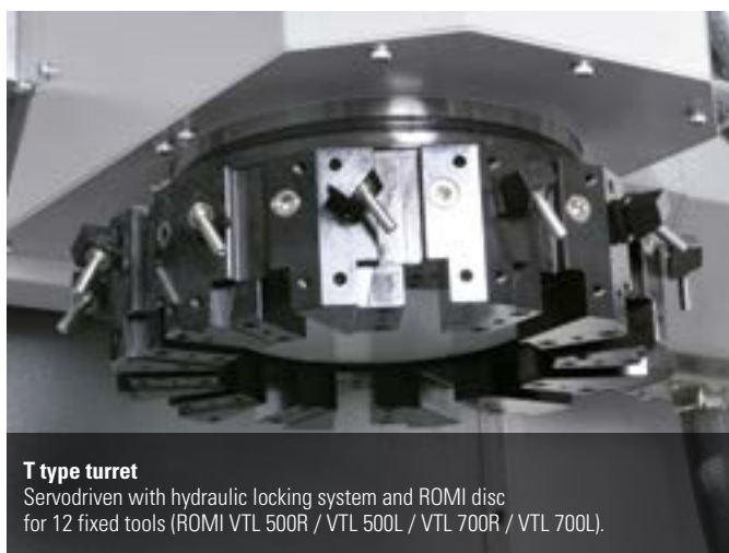
T type turret Servodriven with hydraulic locking system and ROMI disc for 12 fixed tools (ROMI VTL 500R / VTL 500L / VTL 700R / VTL 700L).
