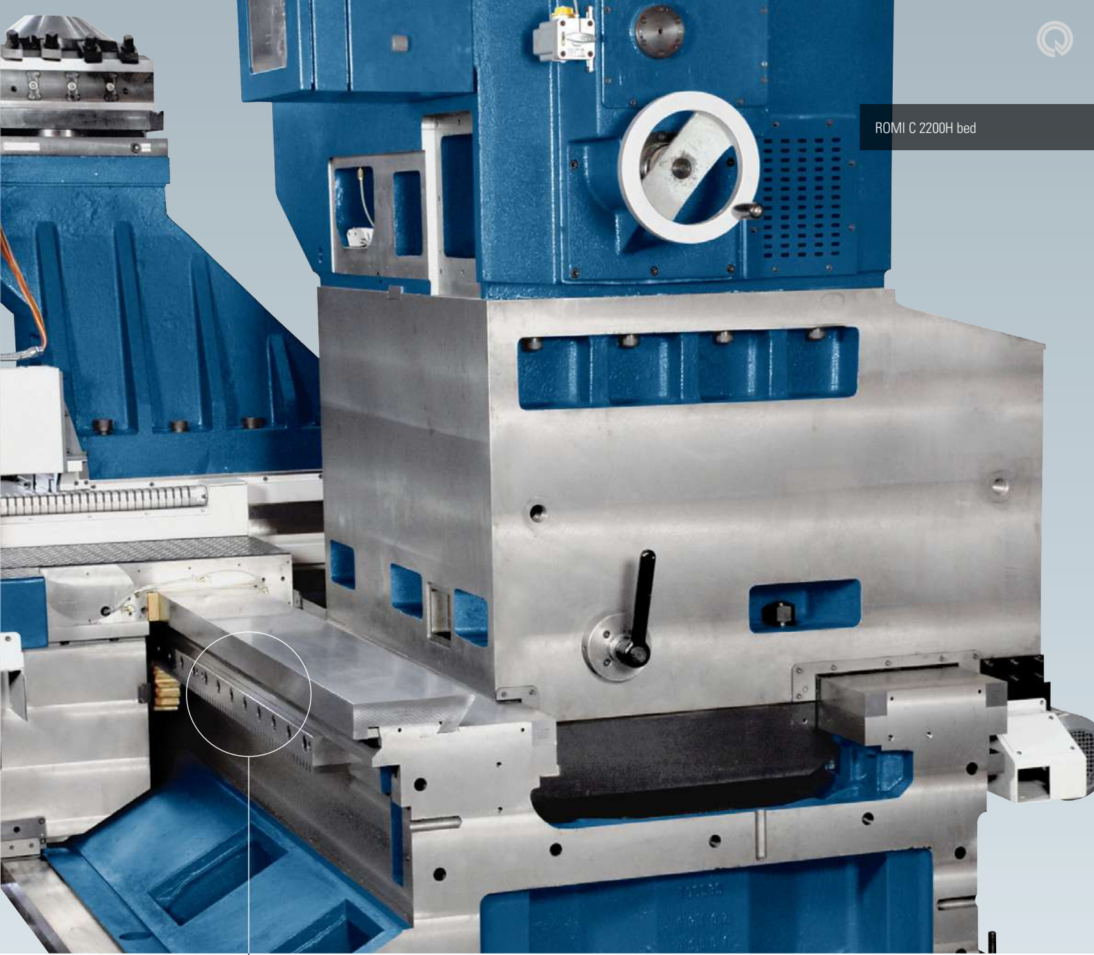
Rack (Güdel) of the longitudinal saddle displacement system.
