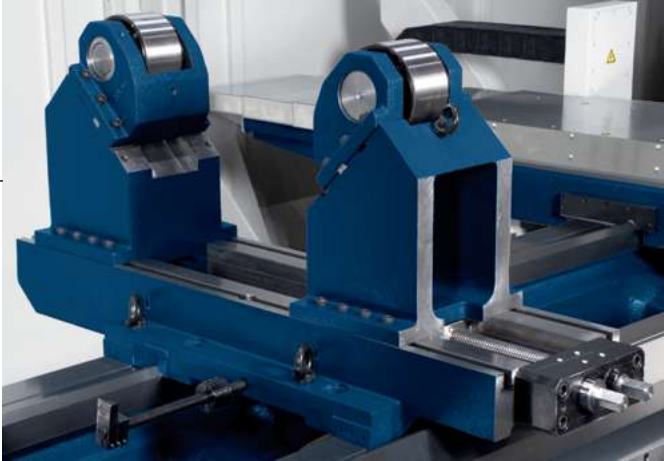
Steady rest C type (optional) Table rest (optional) Equipped with rollers and manual diameter adjustment. It has a drag system via longitudinal saddle for its positioning.
